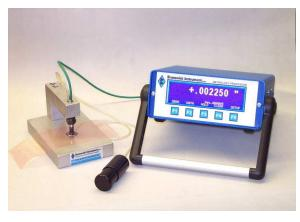
vacuum retract feature. The operator squeezes a hand vacuum pump to lift the probe contact tip before inserting or moving the film sample to prevent stretching or snagging. The probe contact tip supplied has a 1/4" diameter flat with radiused edges for no-snag gaging. Both the probe tip and floating stand anvil are constructed of lapped carbide for extremely long life. A certified .01000" steel gage block is supplied for fast system calibration verification.
