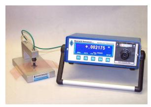
pushbutton, a supplied footswitch, or an external switch closure. A certified .01000" steel gage block is supplied for system calibration verification. A dry, filtered and regulated air supply of 20-60 PSI is required for operation. Air connection is made with a typical 1/4" quick disconnect coupler.
